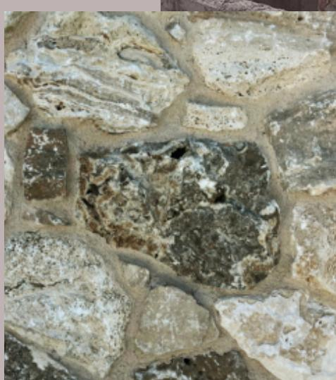
The Antico Nature Rockshell model is created by crushing rubble from the Antico travertine quarry and thinning it down to 2 cm, while preserving its surface form.
