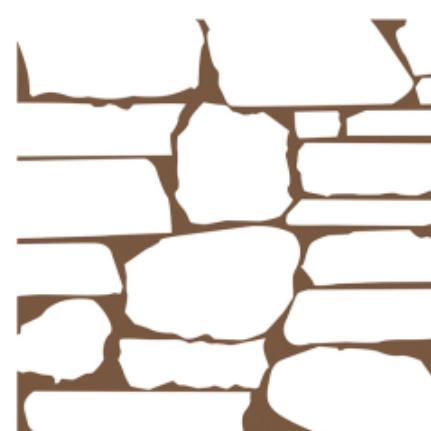
The Mixed Rockshell model is created by mixing unsized, plump stones with stones that are thin and sized in horizontal planes.
